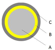
The cross section of the generated multilayer capsule:  $\bf A$  – the hydrophilic core,  $\bf B$  - the middle oil layer, and  $\bf C$  - the polymeric shell.
